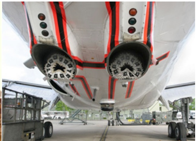
Figure 6. TriStar Tanker HDU signalling lights and testing for AAR alignment markings.
